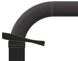
Apply next piece, overlapping and adhering to previous piece by 10mm and ensure that joint will shed water
