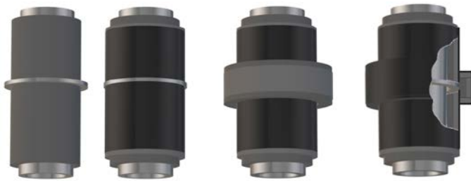
Build up layers of ArmaFlex, ArmaSound RD240 and ArmaSound barrier
