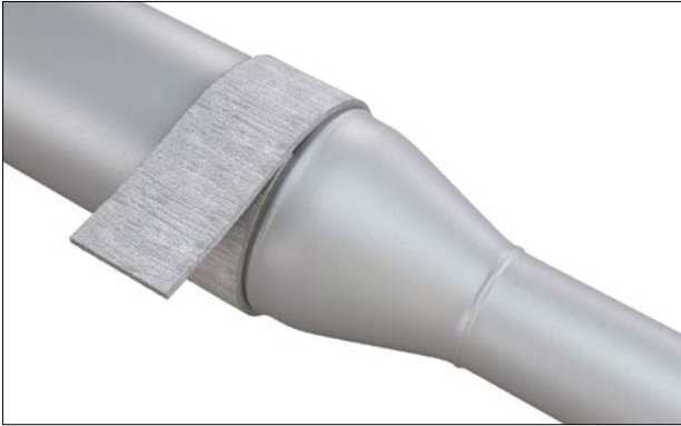
Figure 45: Measuring pipe circumference.
