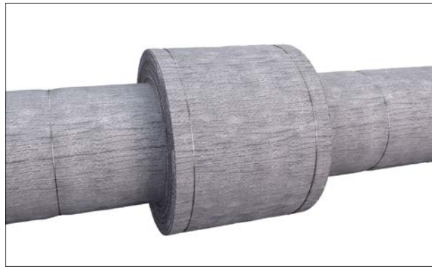
Figure 33: Securement of flange insulation cover.
