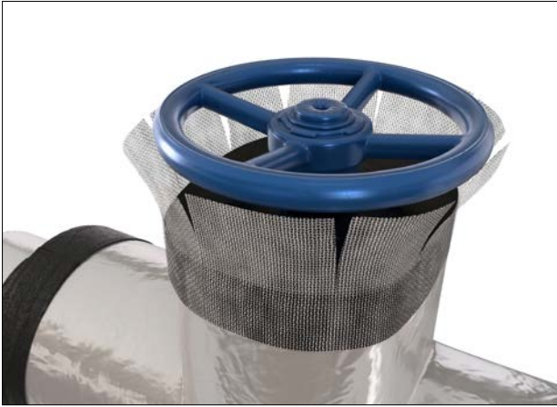
Figure 56: Application of the flexible reinforcing membrane at spindle insulation termination
