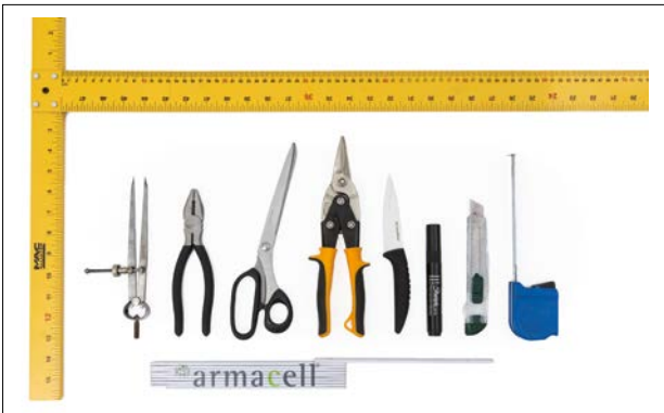
Figure 4: Recommended tools for application of ArmaGel DT
