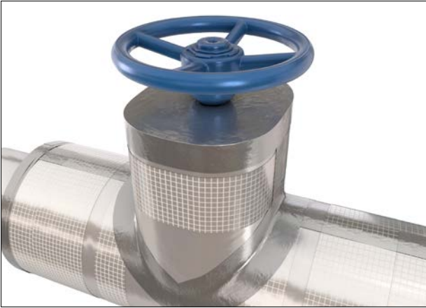
Figure 51: Application of vapour barrier tape at all joints and seams
