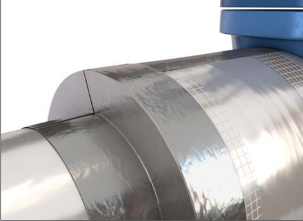
Figure 46: Completely sealed termination
