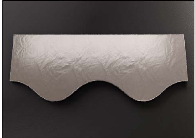
Figure 48: Fabricating the insulation for valve connection
