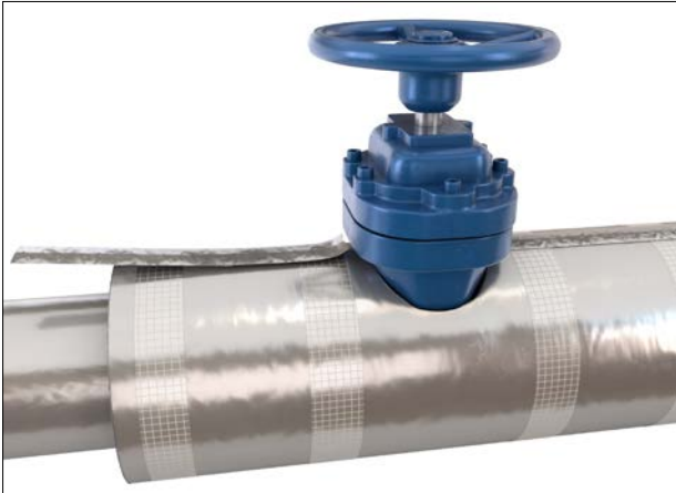
Figure 42: Application of vapour barrier tape
